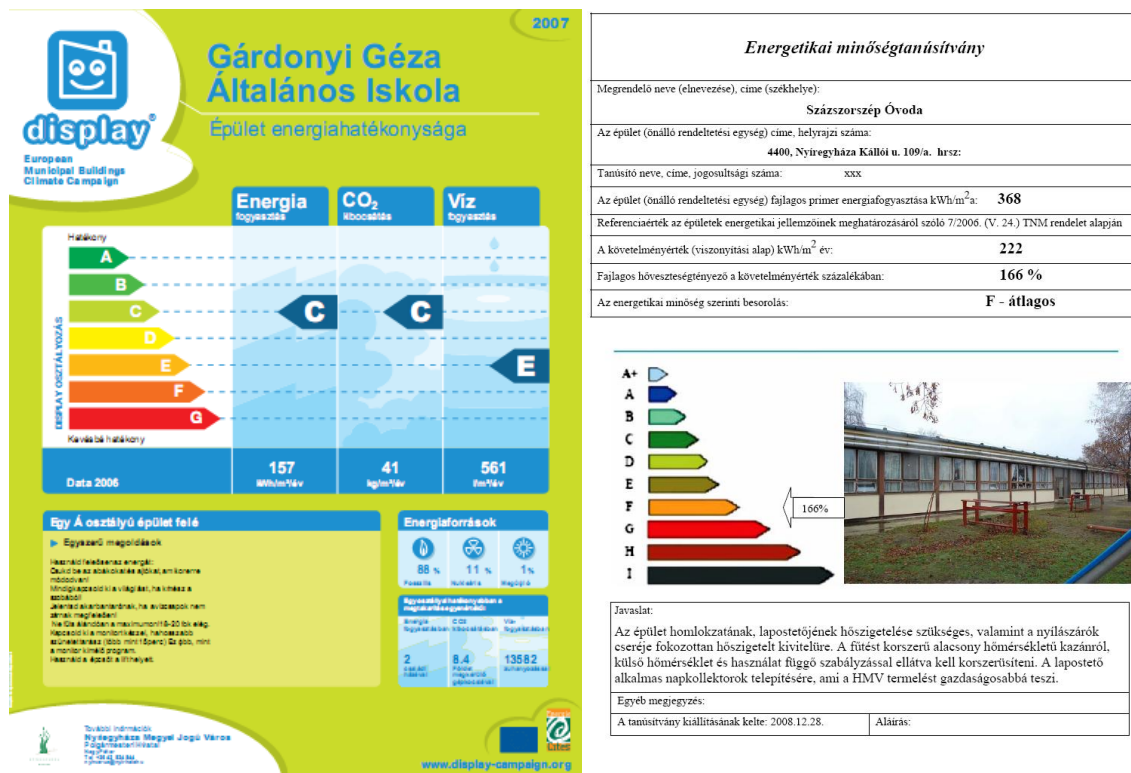
Figure 1: The Display label and the energy certificate specified in the Government Decree (credit: Péter Nagy)
